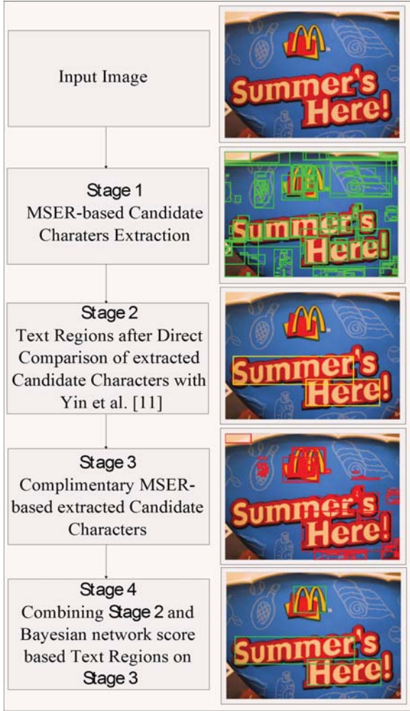
Fig. 1. Flowchart of Stage Wise Text Detection in Scene Images
